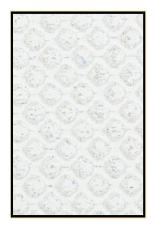
Figure 3. Type III Preformed Plastic Tape
