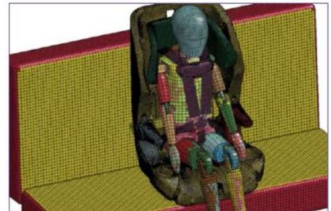
Hybrid III 6-year-old ATD in a forward-facing child restraint on the C/FMVSS bench in a finite element simulation
