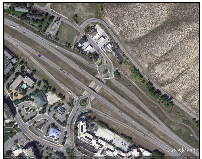
Figure 2-20. Aerial Photo of a Two-Level Roundabout Interchange with a Figure-8 Roundabout in Avon, Colorado
