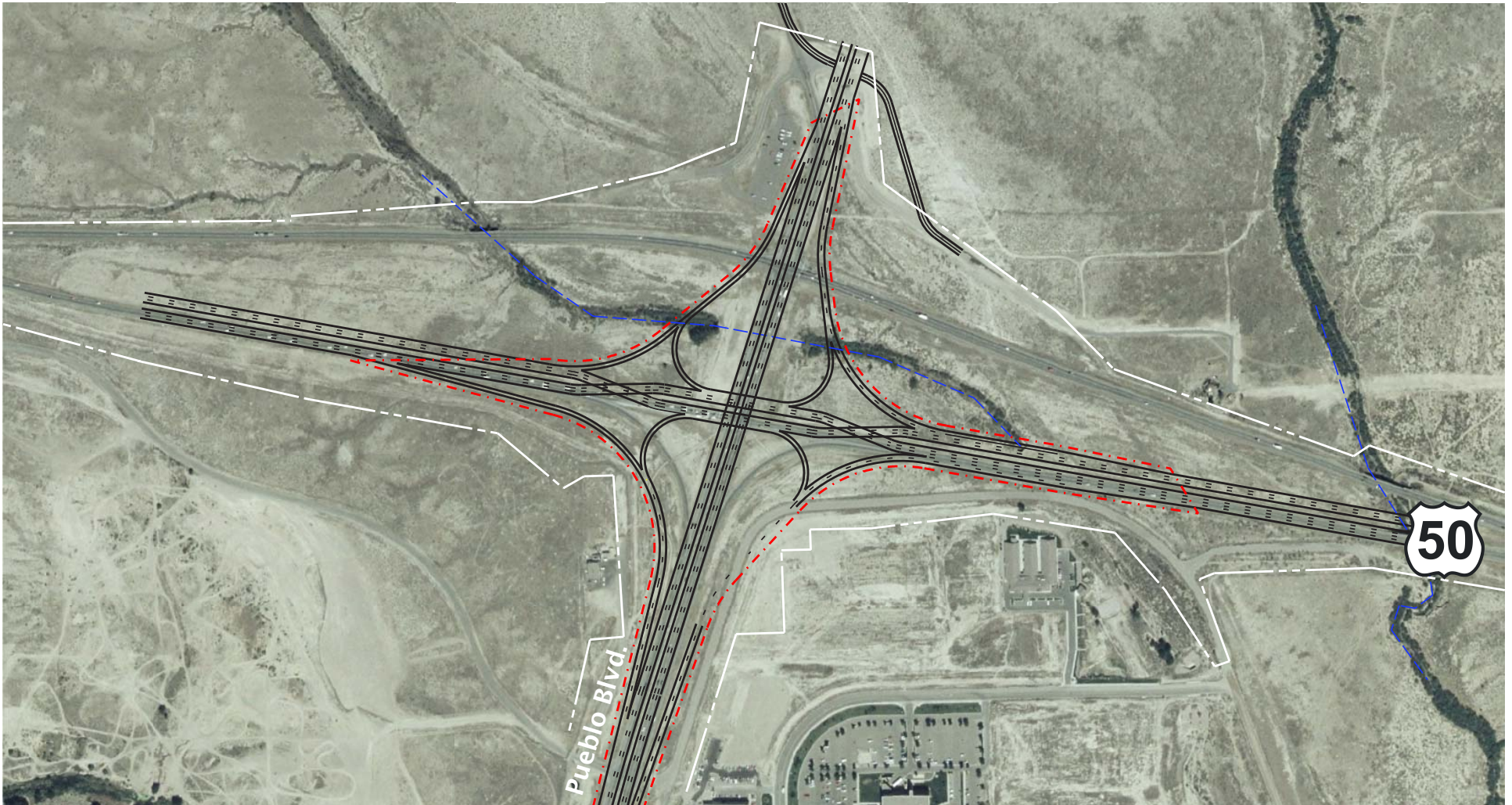
Figure 2-31. Aerial View of Diverging Diamond Interchange at Pueblo Blvd.
