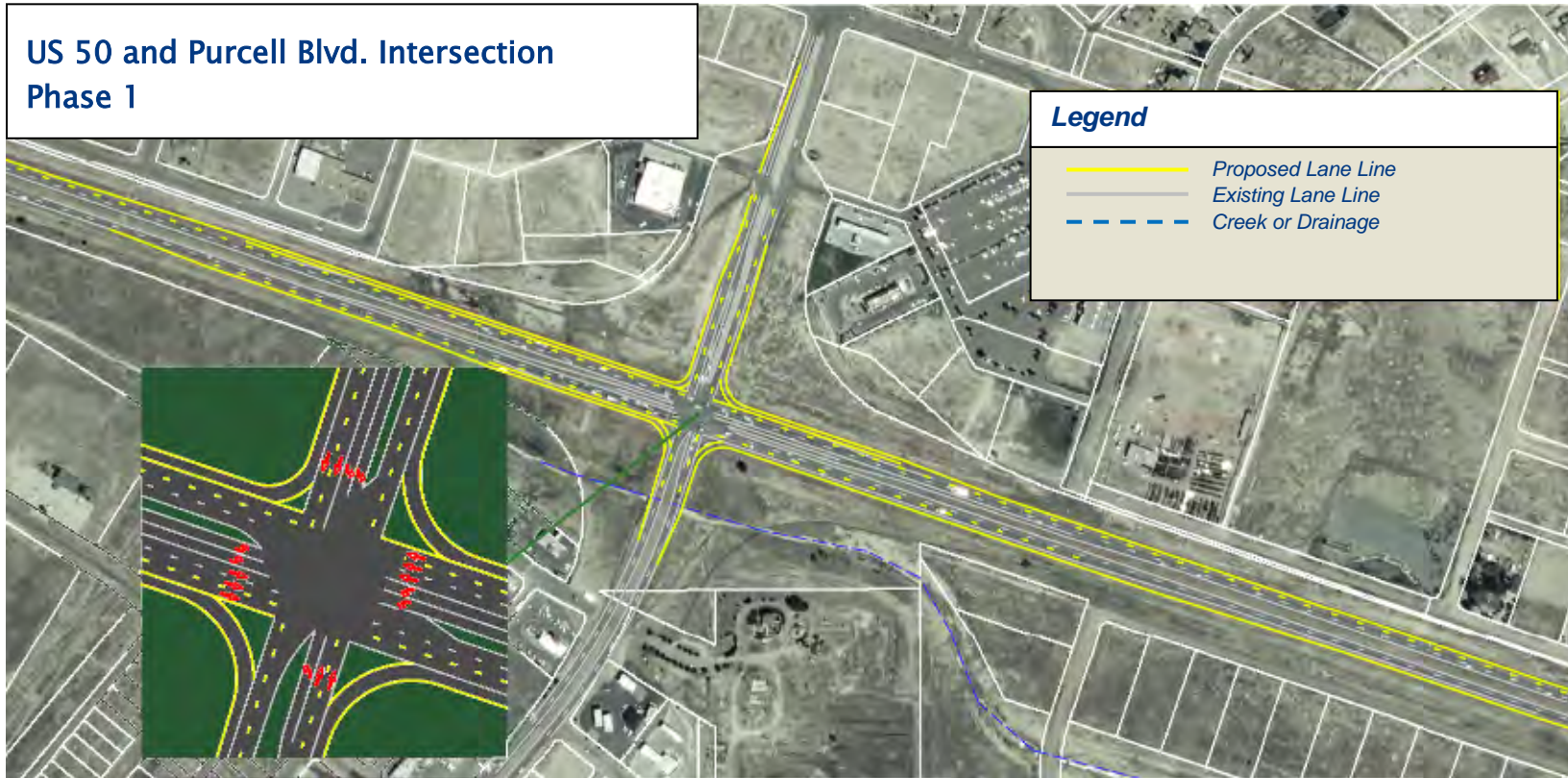
Figure IP-8. Phase 1 Improvements at US 50 and Purcell Blvd.
