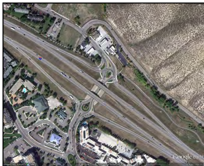
Figure 2-20. Aerial Photo of a Two-Level Roundabout Interchange with a Figure-8 Roundabout in Avon, Colorado
