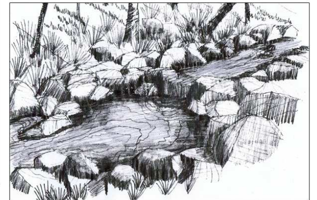
D | Drop structure using indigenous rock construction.
