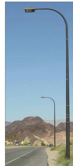
B | Light poles should be of an elegant and simple design with full-cutoff luminaire fixtures. The image on the left is an ideal example.
