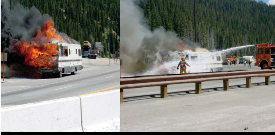
Tunnel Pumper Deluge System with Foam
