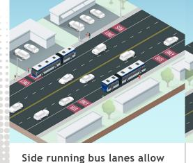
buses to move through the corridor without delays from general traffic congestion. Right-turning vehicles are allowed to use the bus lane to turn right.
