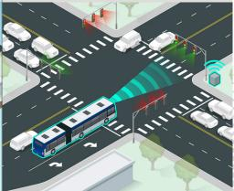
Transit signal priority allows buses to communicate with traffic signals as they approach an intersection. This allows the bus to proceed through an intersection more efficiently.
