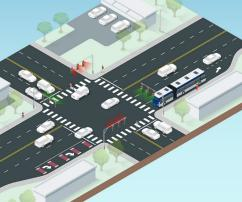
Bypass lanes and queue jumps are located at targeted intersections where buses typically experience significant delay. They provide priority to buses to reduce delay experienced.
