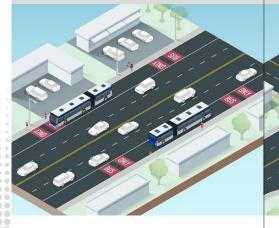
Side running bus lanes allow buses to move through the corridor without delays from general traffic congestion. Right-turning vehicles are allowed to use the bus lane to turn right.
