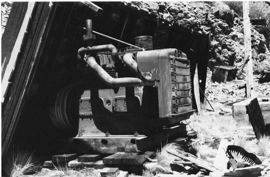
The V-cylinder compressor, similar to a large engine, became one of the most popular compressor types during the 1930s. Note the foundation. Source: Eric Twitty.
