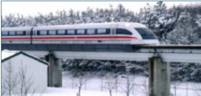
Transrapid is German developed system, commercially available in Shanghai, with a lower cost than steel-wheel trains with tunnels. Also, it can climb steeper (7%) grades.
