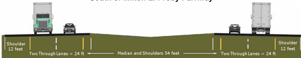
Exhibit 3-9. Lane Configuration for 4-Lane Freeway South of Milton E. Proby Parkway
