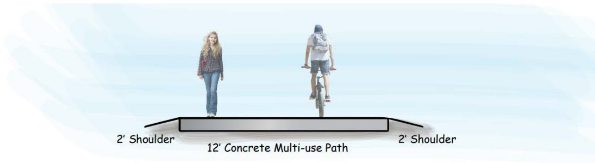
Figure 4-4. 2 Shared-Use Path Typical Section
