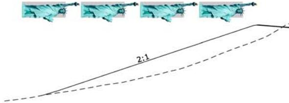
THIS DETAIL HAS BEEN SCALED DOWN TO SHOW WHAT THE IMPACTS WOULD BE WITHOUT WALLS AND USING A 2:1 SLOPE. THE SLOPE WOULD NOT CATCH UNTIL ABOUT 600' OR 4 STATUE OF LIBERTIES LAYING END TO END.
