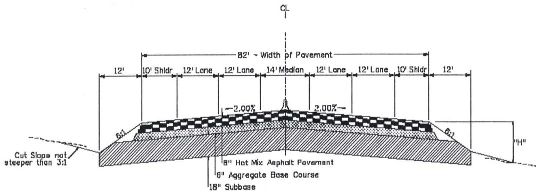
Figure 1: Typical Section of roadway used for this analysis
