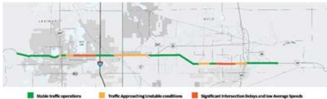
Figure 4-6. Quality of Traffic Flow During Peak Periods Corridor Existing Conditions Report US 34 PEL
