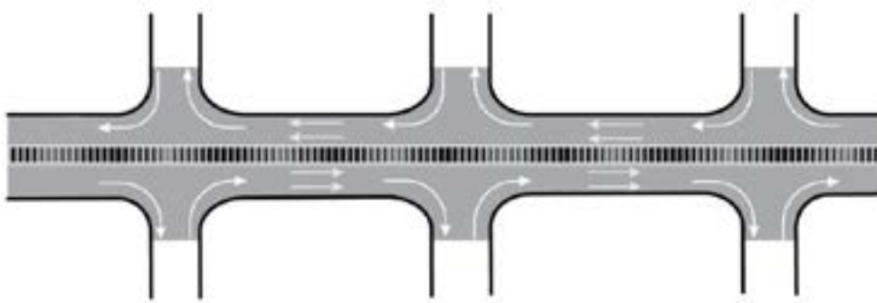
Figure 5-5. Install Medians and Islands
