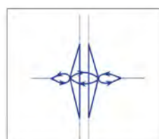
Diverging Diamond Interchange
