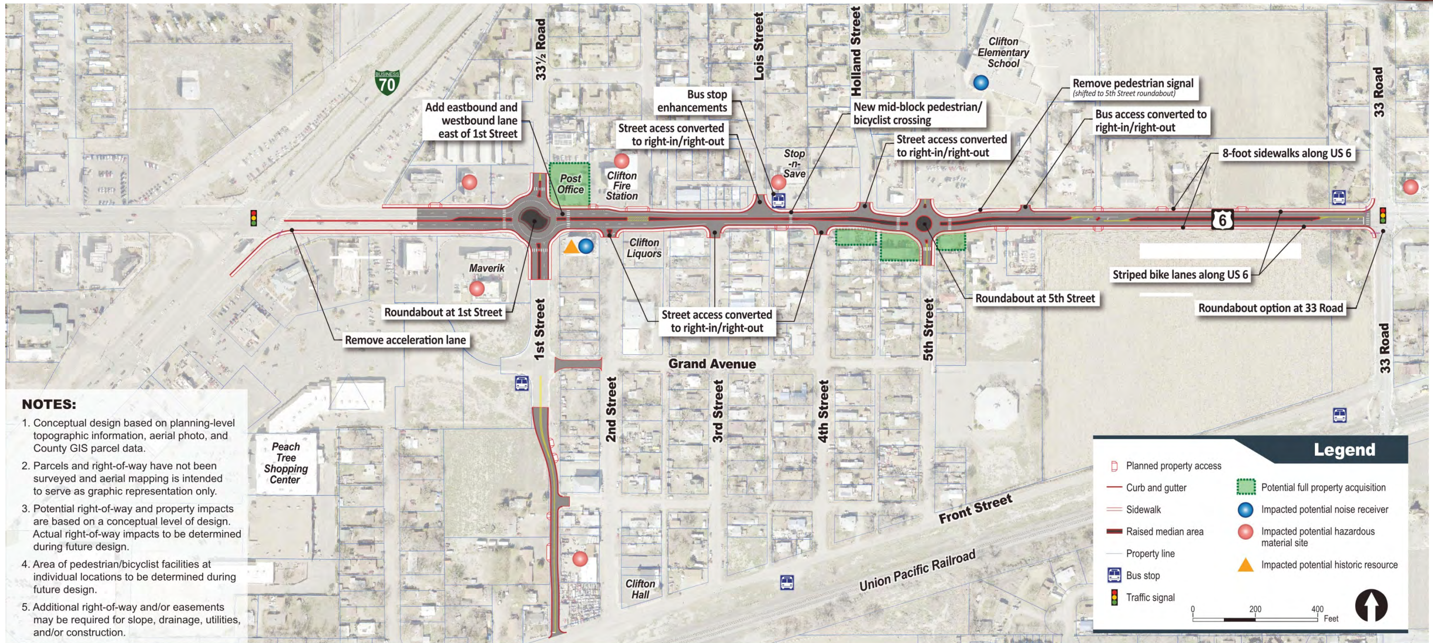
Figure 14: Alternative 1 – US 6 Improved Two Through Lanes, Option B - Roundabouts
