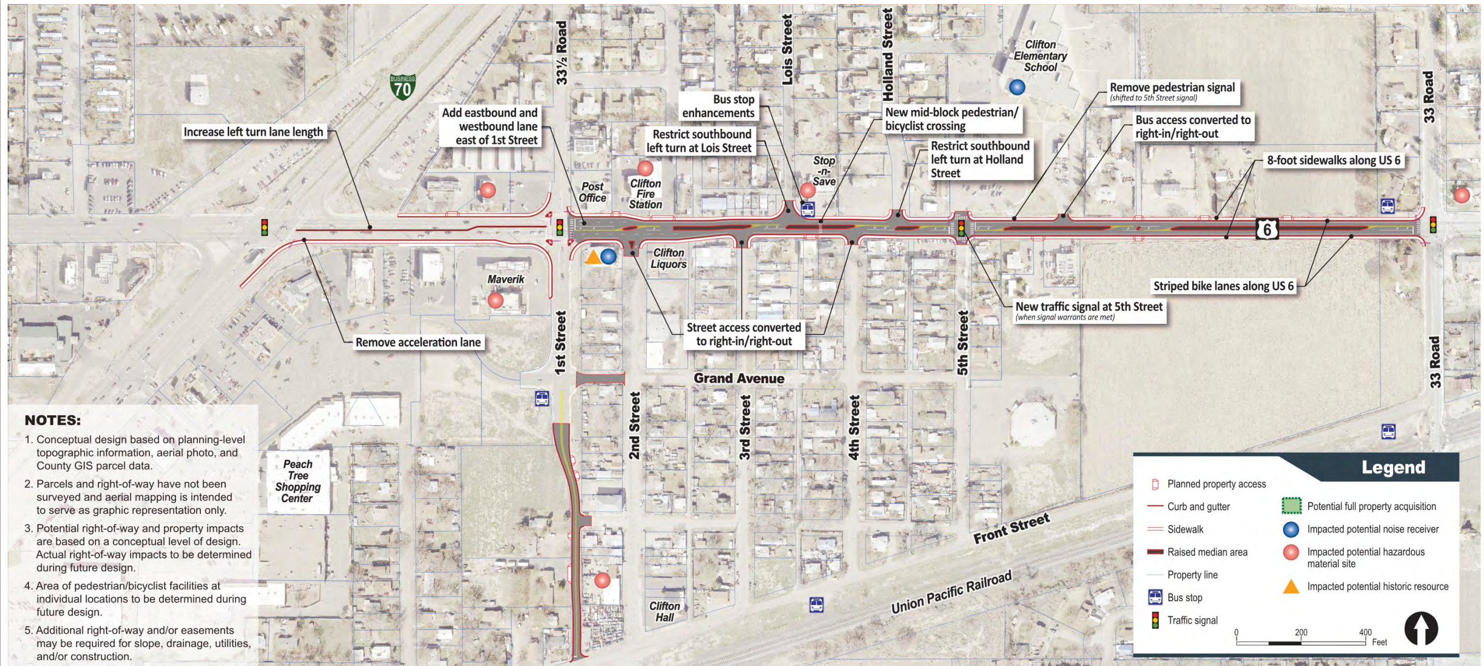
Figure 13: Alternative 1 – US 6 Improved Two Through Lanes. Option A - Traffic Signals
