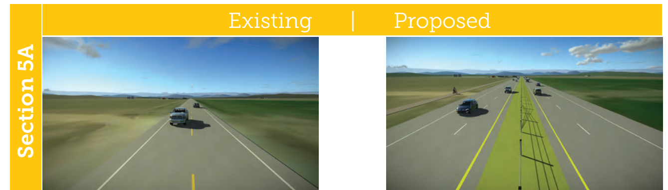
No median separation or left turn lanes
