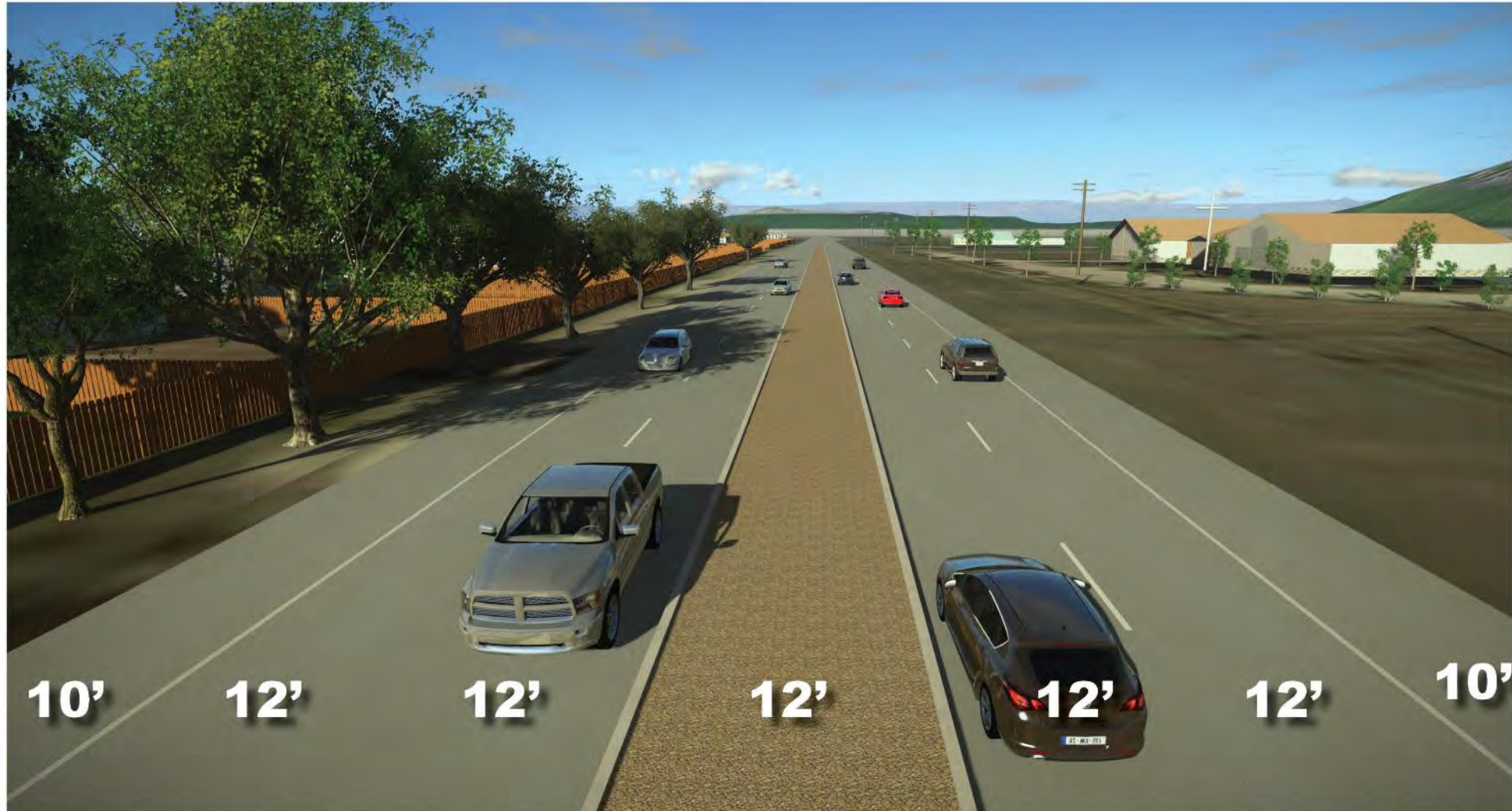
Section 2 - Proposed roadway conditions
