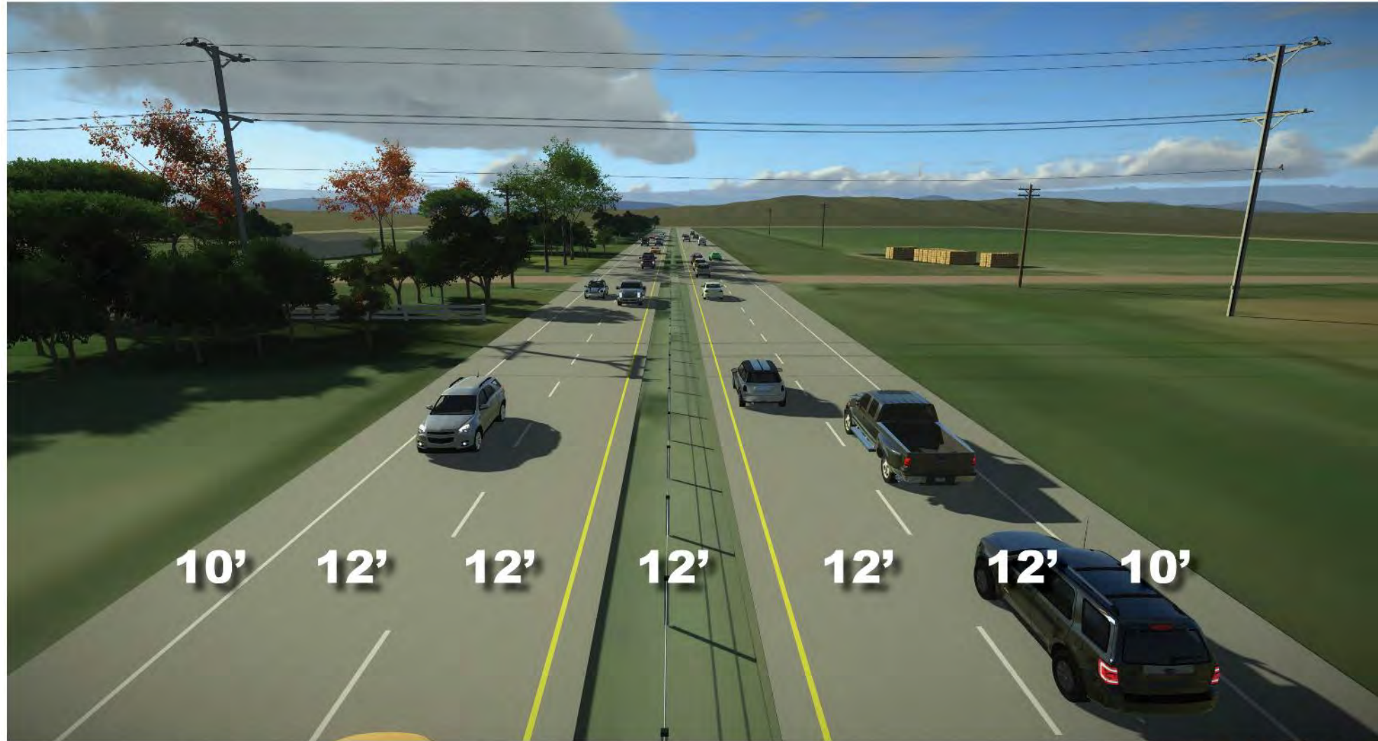
Section 3 - Proposed roadway conditions
