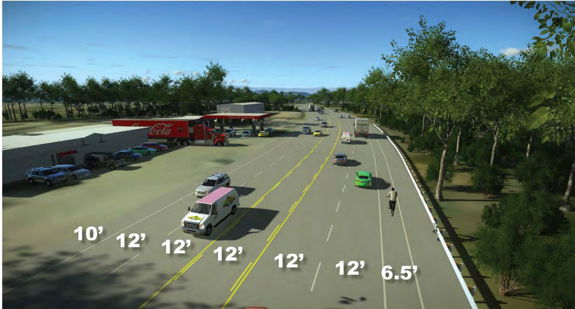
Section 1A - existing roadway conditions
