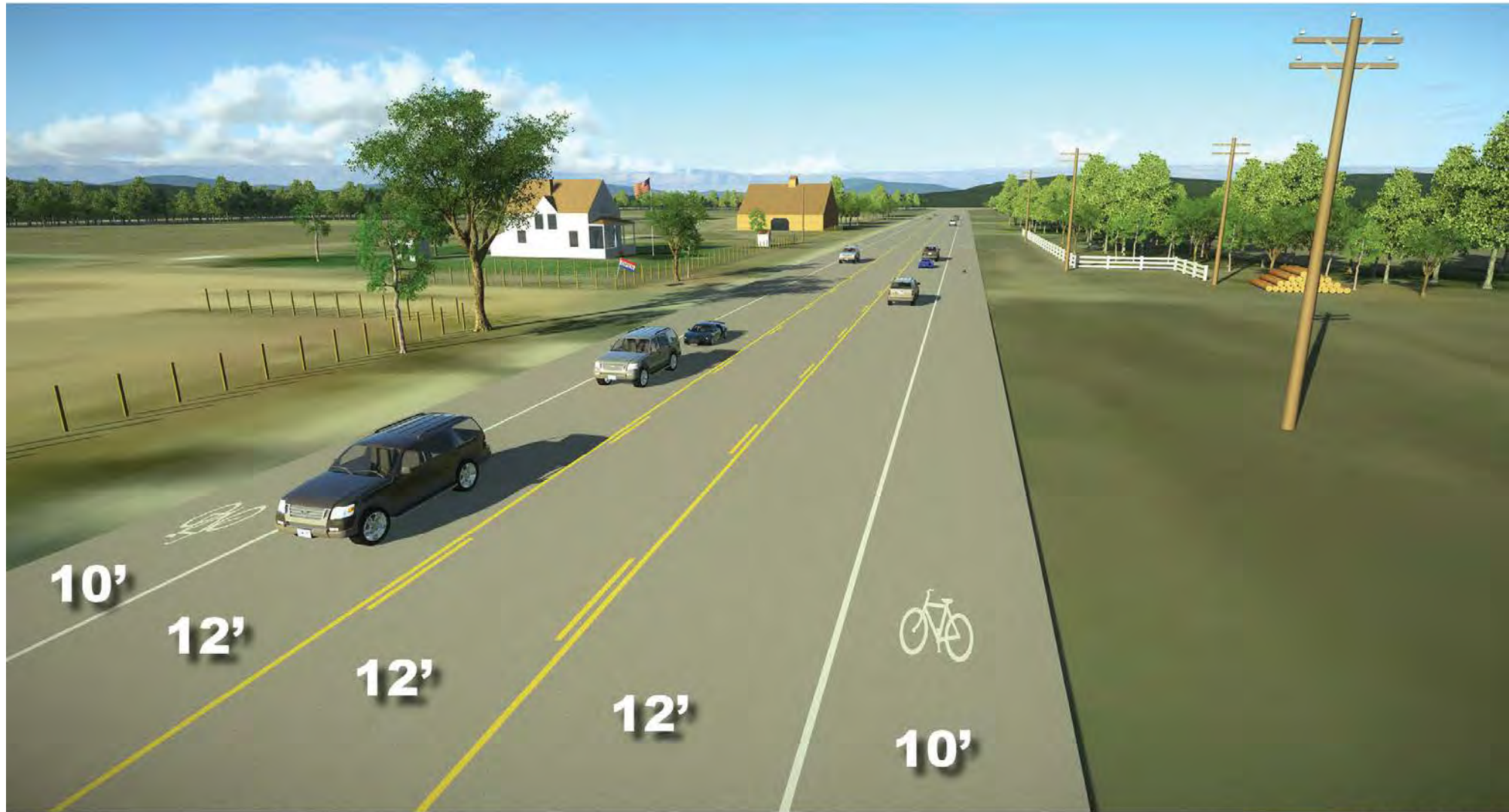
Section 1C - Proposed roadway conditions
