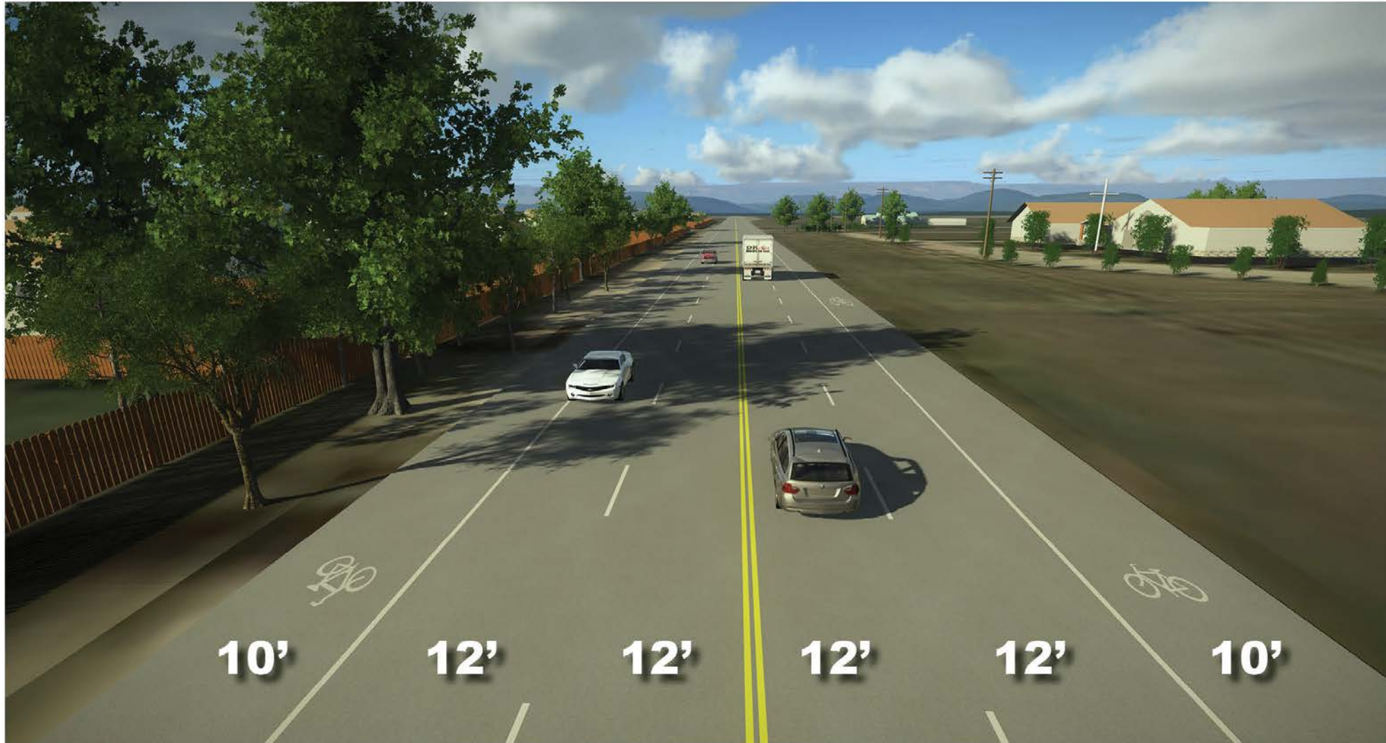
Section 2 - Proposed roadway conditions
