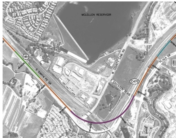
Exhibit 3-26: From Median of Santa Fe, elevated Alignment over Northbound Lanes, County Line Road, Two Railroads, C-470, and the Santa Fe/C-470 Flyover Ramp
