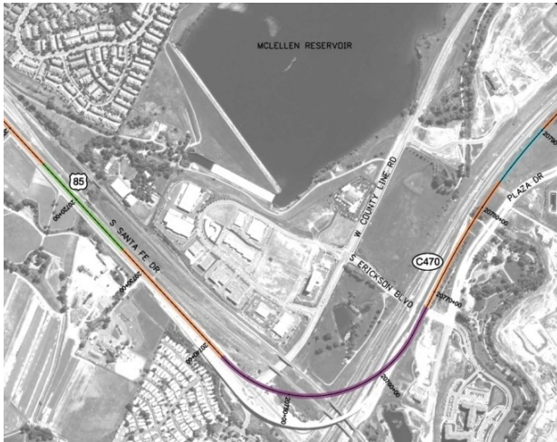
EXHIBIT 5-35: FROM MEDIAN OF SANTA FE, ELEVATED ALIGNMENT OVER NORTHBOUND LANES, COUNTY LINE ROAD, TWO RAILROADS, C-470, AND THE SANTA FE/C-470 FLYOVER RAMP
