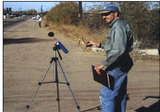
Figure 2-57. Measuring sound levels on a roadway near downtown Colorado Springs.
