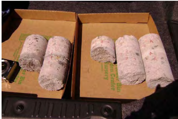
Figure 3-4 Coring samples on Bridge G-22-BH
