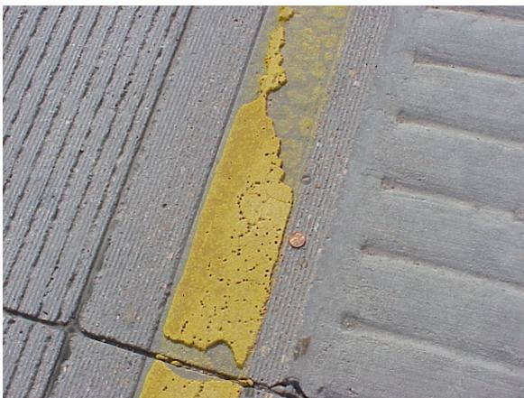
**Figure 7. The thermoplastic failed due to adhesion loss.**
