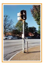
Curb Extensions. Appropriate at intersections where an on-street parking lane exists, curb extensions extend
