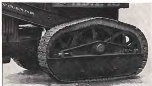
Furnished with semi-crawlers for soft going and heavy maintenance on dirt roads
