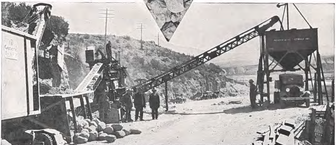
No. 22-B Pioneer Screening, Crushing and Loading Plant—screens, crushes and loads all in one operation—capacity 200 to 350 cubic yards in 10 hours, based on one-inch reduction and 25% oversize. Plant has chain drive, SKF bearings, and mechanical feeder. A 21-yard Pioneer Storage Bin is also part of above hook-up. This equipment was furnished by Elton T. Fair, Pioneer Distributor in Denver, Colo., to Delta County, Colo., and is in operation near Hotchkiss, Colo.
