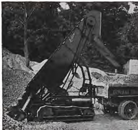
Below: McCormick-Deering-powered loader used for loading construction materials, for digging and loading dirt in road building, and for snow-removal work.
