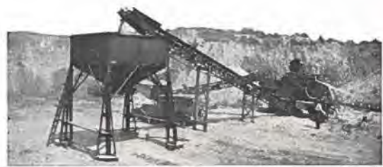
No. 22B Pioneer Screening, Crushing and Loading Plant, equipped with No. 824 Universal Jaw Crusher, owned by St. Joseph Co., South Bend, Ind. Capacity, 250 to 700 cubic yards per day, depending upon oversize. An ideal plant where pit-run gravel does not contain too much oversize.
