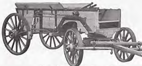
Stroud Contractor's Dump Wagon.
