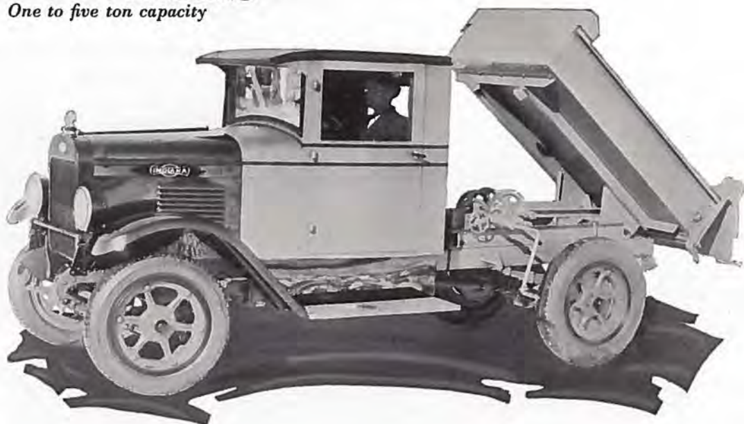
Indiana Model 111—1½-Ton Chassis With Hand Hoist and Dump Body
