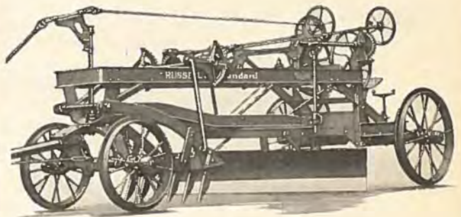
8-foot Blade. Weight: With Scarifier, 4,775 lbs. Without Scarifier, 3,500 lbs.
