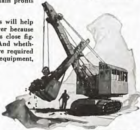
Replacing the crane boom with shovel boom is a matter of only a few hours. The powerful crowding motion is an exclusive P & H development.
