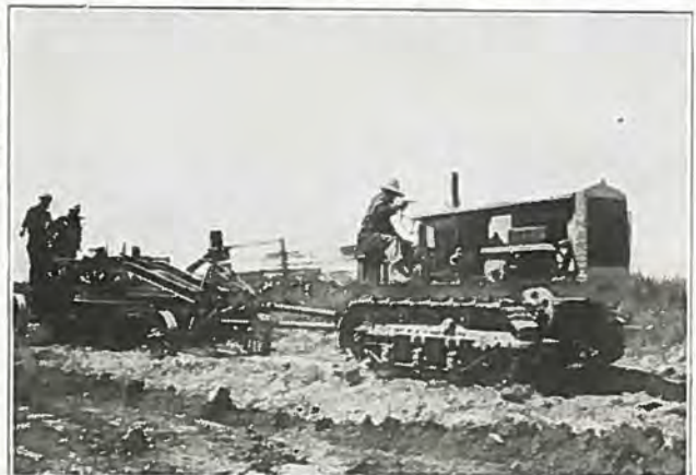
"30" Monarch Pulling 10-ft. Grader THREE FORWARD SPEEDS A GIANT FOR PULLING
