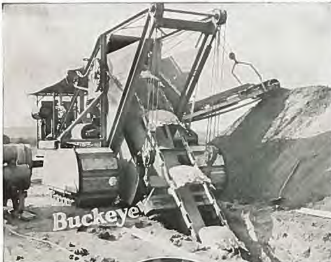
The Rotary Auxiliary Cutter may be attached to any chain and bucket type Buckeye. It increases the cutting range to almost any width. Requires no extra power.
