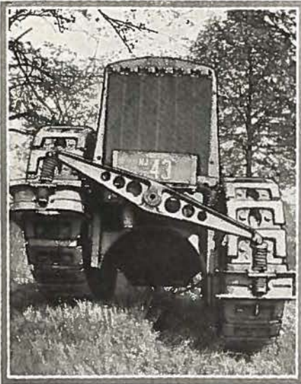
Showing flexibility of Bear tractors as used in side-ditch of road
