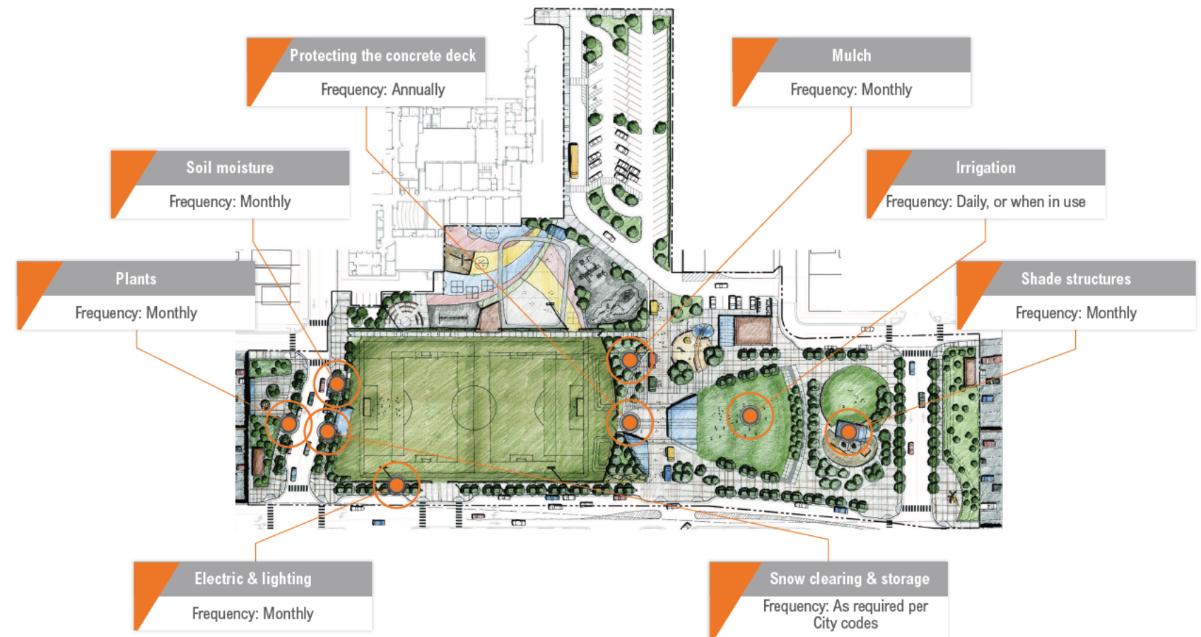
Figure 5.21 | Elements Requiring Inspection and Maintenance: We will document installation of all items needing inspection in accordance with the record keeping requirements of the cover top O&M work.
