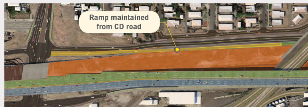
The newly constructed CD Lane will push traffic through the newly constructed lowered section approach to Brighton Boulevard. The off-ramp will be maintained at all times during construction to allow for demolition of the Brighton Boulevard WB off-ramp and construction of the approach to the bridge.
