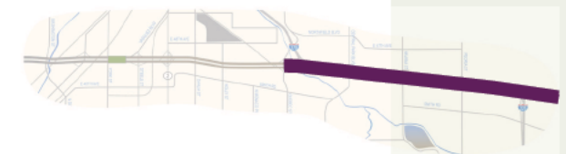
Figure 3.11 | Schematic of Work Area 1, Sand Creek to Chambers: This "inside-out" approach involves full reconstruction of the Peoria Street interchange, demolition and construction of a new flyover structure at the I-70/I-270 interchange, outside widening from STA 2194+00 to 2379+00 with resurfacing of existing pavement, replacement of the median barrier and lighting system, and restriping/signing of the I-225/I-70 interchange.
