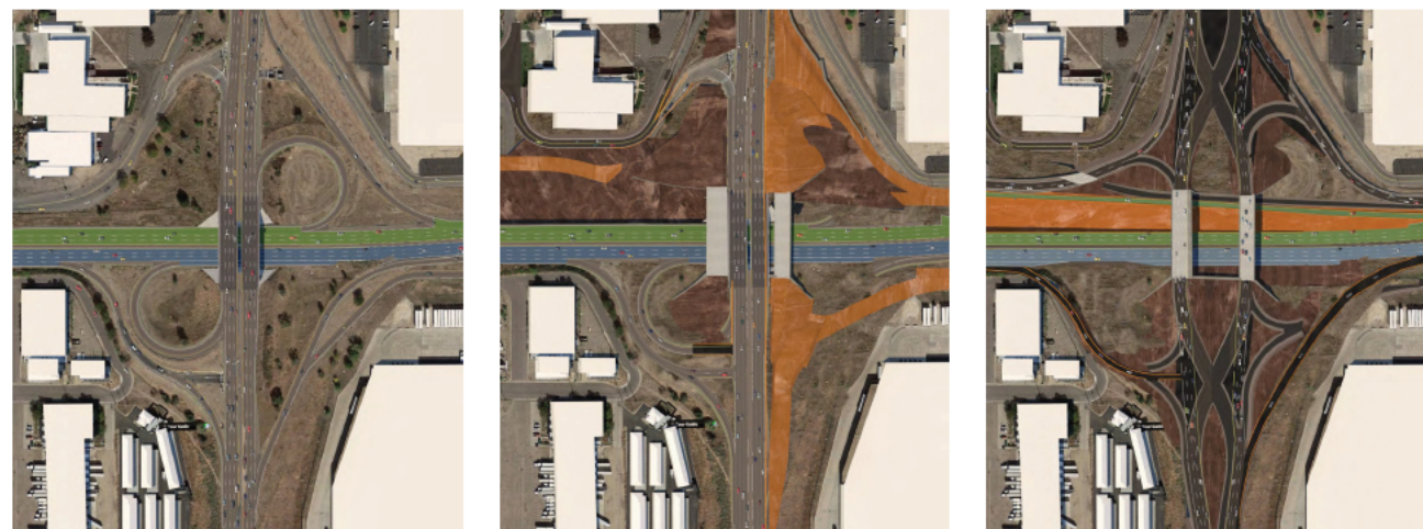
Figure 3.16 | Schematic of ATC 2, Diverging Diamond Interchange at Colorado Boulevard: 5280 Connectors developed a dynamic innovation by using a diverging diamond interchange (DDI) to benefit the project during and after construction.
