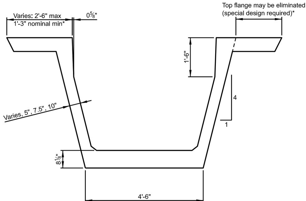
\*When setting the top flange width of U girders, the Designer shall consider the loss of concrete width for interface shear resistance due to the support requirements for partial depth precast deck panels. While the top flange of U girders may be eliminated entirely from a fabrication standpoint, the limited remaining interface width may preclude using partial depth precast deck panels.
