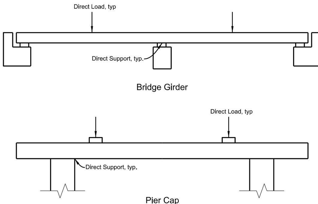
**Figure 5-9: Examples of Direct Supporting and Loading Conditions**
