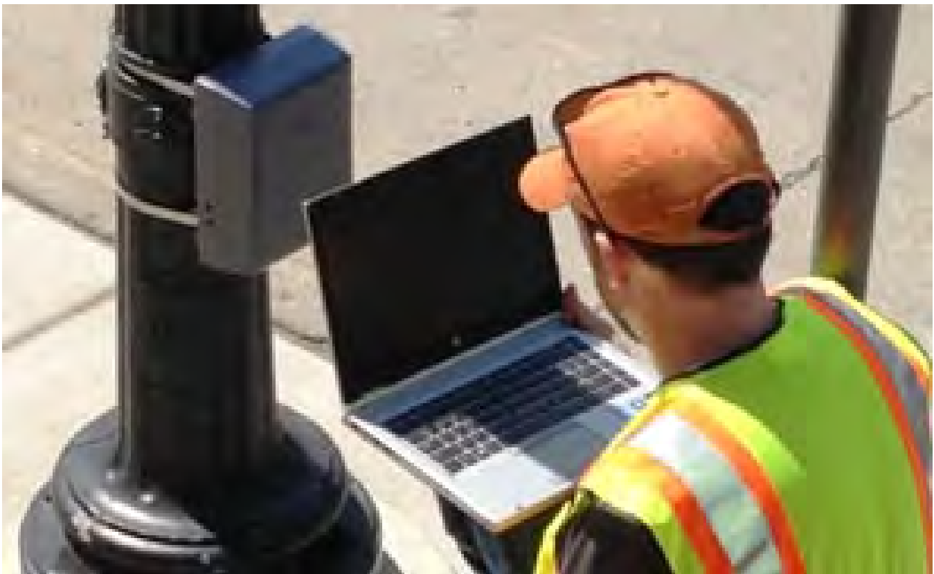
Figure A-3. Field Data Collection from a Passive IR Counter
