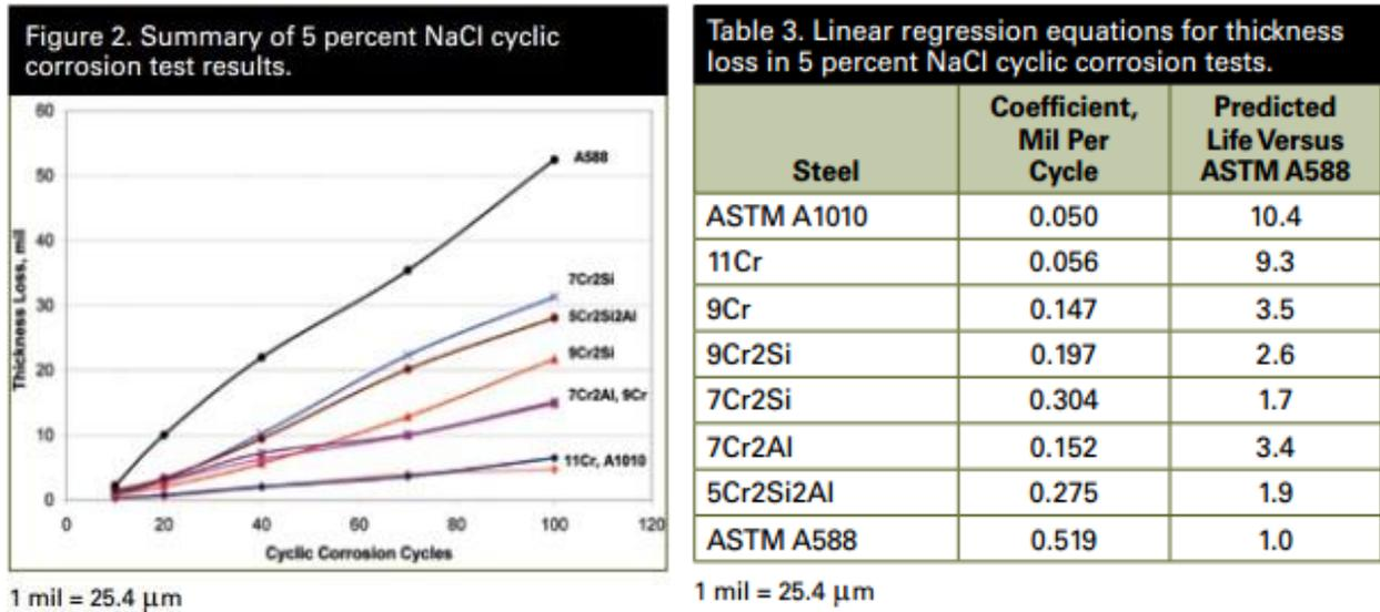
Figure 1 - Results of Corrosion Tests on Steel Alloys
