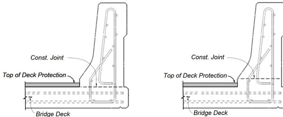
**Figure 2 - Alternative Construction Joint Placement of Deck/Barrier Interface**
