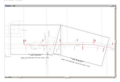
15. Select the plan sheet border cell **SHEET\_ROW-Plan-Sheet** for ROW and Survey or select **SHEET\_Design-Sheet** for all other disciplines from the **General** cell library.
