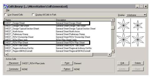
16. Place the sheet border cell so the lower-left corner coincides with the corner indicated on the sheet limits cell previously placed. Set the **Active Angle** and the **Active Scale** to the same value that is indicated in the Sheet Plan Limits cell.
