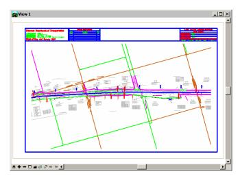
**Note:** Rotating a MicroStation view simply rotates the viewing of the graphics. The coordinate system is still relative to the graphics and any coordinate or alignment information extracted will be correct.
