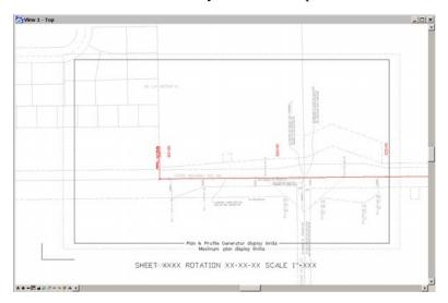
7. Use the **Edit Text** command to update the text at the bottom of the sheet. This will assist in managing the sheet plan limits.
