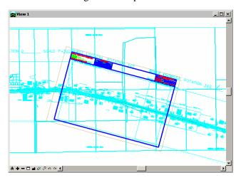
Rotate the MicroStation view so that the sheet is normal to the view
