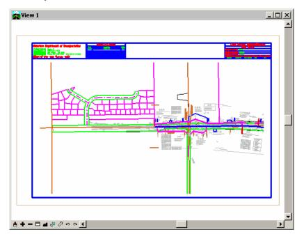
Using the tentative (snap) button on the mouse to query coordinates reports values that correctly reflect project coordinates. Additionally an InRoads command, such as tracking, will verify the graphics are coordinately correct.
