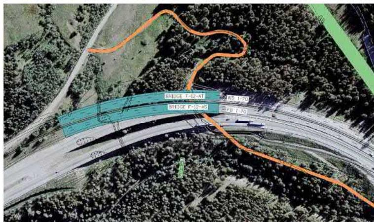
Proposal 9: Build new WB bridge where designed and put WB traffic on it, then use existing WB bridge for EB traffic and build new EB bridge on existing location at Miller Creek.
