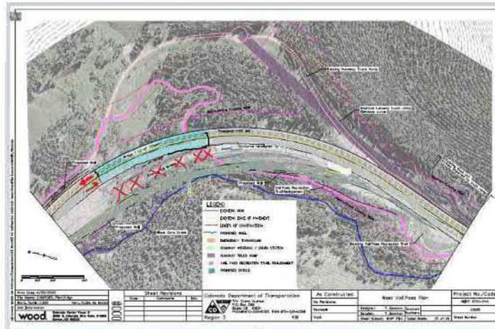
Proposal 8: Build new WB bridge where designed, demo existing WB bridge and construct EB bridge in the same location at Polk Creek.
