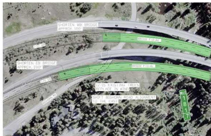
Proposal 2: Construct both bridges to the north of existing bridges at I-70 crossing of Big Horn and Gore Creek in EA area.
