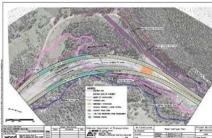
Proposal 8: Build new WB bridge where designed, demo existing WB bridge and construct EB bridge in the same location at Polk Creek.
