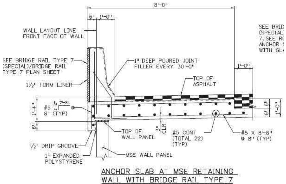
*Example Anchor Slab Detail*
