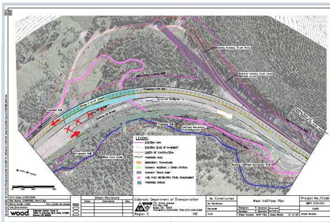
Once the new WB bridge is complete, WB traffic is shifted on to it. The existing WB bridge is demolished and a new EB Bridge is constructed parallel to it. EB traffic remains on its existing bridge.
