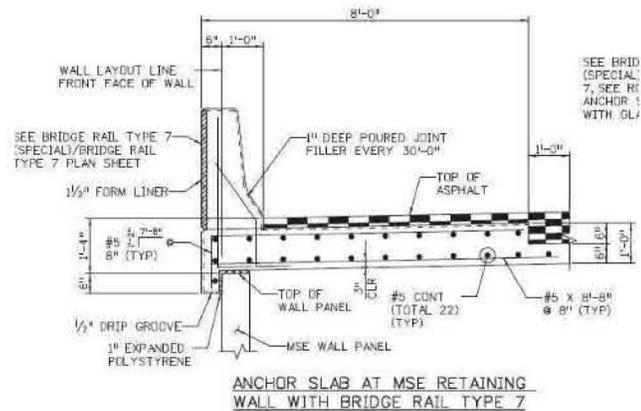
Example Anchor Slab Detail
