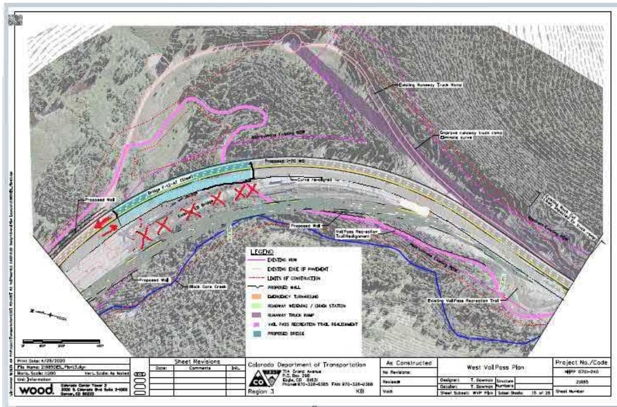
Once the new EB bridge is complete, EB traffic is shifted on to it. The existing EB bridge is demolished.
