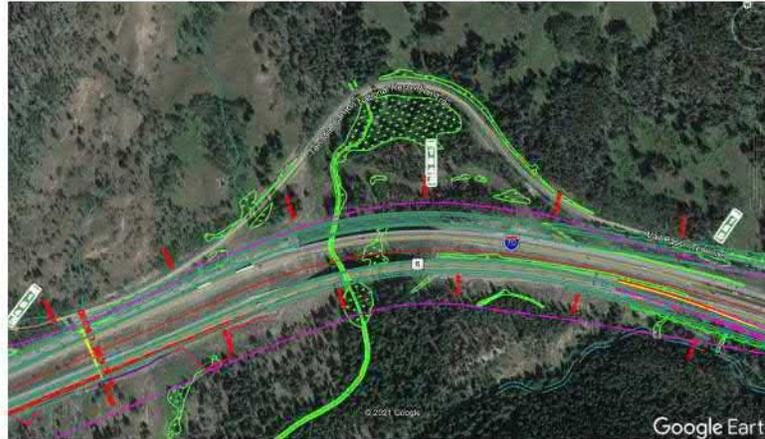
Proposal 10: Consider relocating improved truck parking to eliminate a retaining wall at the top of the hill near MP 190 or eliminate completely.
