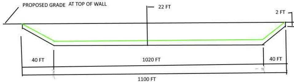
$$\text{Area of wall} = 2 \times 1100 \text{ FT} + 20 \times 40 \text{ FT} \times 2 / 2 + 1020 \text{ FT} \times 20 \text{ FT} = 23,400 \text{ SQ FT}$$
