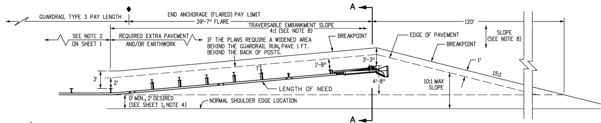
**PLAN VIEW WIDENING FOR END ANCHORAGE (FLARED) \***
