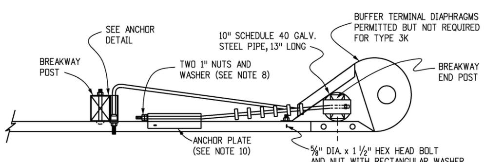
**LOW SPEED END ANCHORAGE - TYPE 3K**
