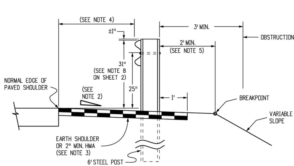
**NORMAL ROADSIDE INSTALLATION WHEN FILL REQUIRES GUARDRAIL**
