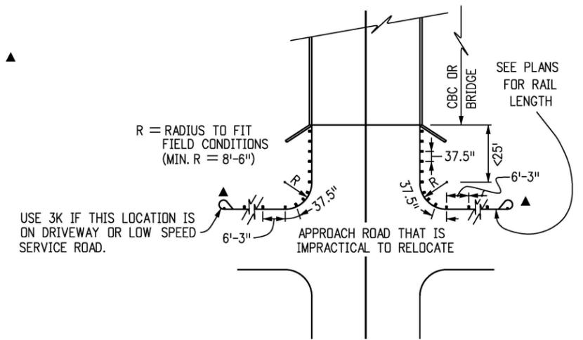
GUARDRAIL TYPE 3 WITH BLOCKED OUT POSTS SPACED AT 3'-1/2" FROM STRUCTURE AROUND CURVE.
