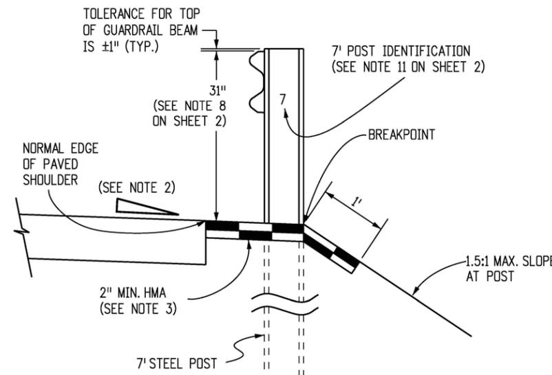
**RESTRICTIVE ROADSIDE INSTALLATION WITH 7 FOOT GUARDRAIL POSTS**
