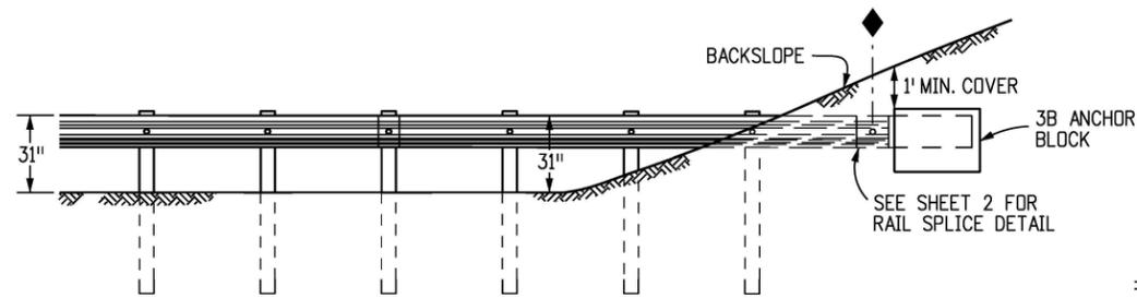
SEE TYPE 3B (RUB RAIL) PLAN VIEW FOR ALIGNMENT. THE 100 FT. FLARE LENGTH MAY BE SHORTENED IF THE SLOPE IS LESS THAN 8 FT. WIDE.
