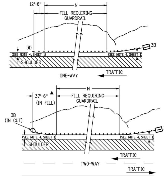
**GUARDRAIL FOR ROADSIDE CUT-TO-FILL CONDITION**
