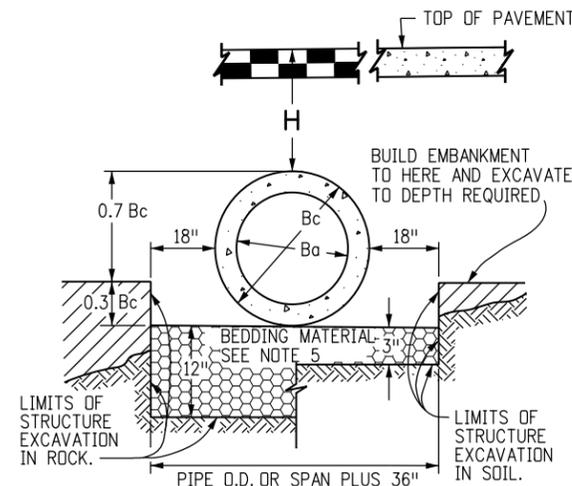
NOTE: Bc IS THE OUTSIDE DIMENSION FOR DIAMETER, SPAN OR RISE.
