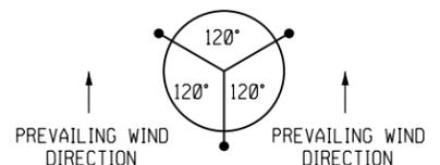
NOTE: FOR TREES ON 4:1 OR STEEPER SLOPES, PLACE TWO GUYS UPSLOPE AND ONE DOWN SLOPE. OTHERWISE, PLACE FOR PREVAILING WIND.
