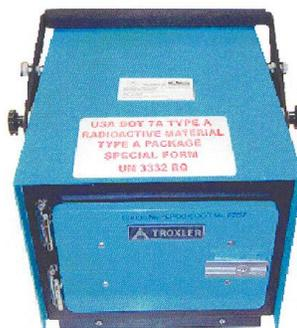
Troxler 3241-C Asphalt Content
