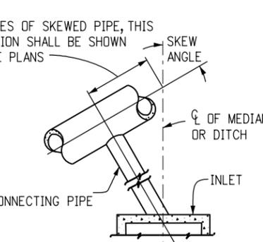
**INLET CONNECTED TO A SKEWED CROSS PIPE**
