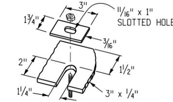
**ALTERNATE SLOT AND HOLD DOWN PLATE DETAIL**
