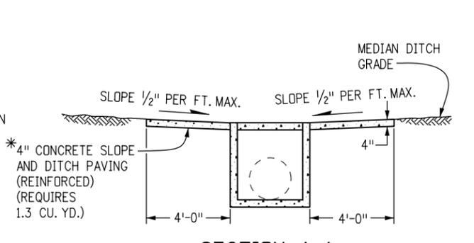
**SECTION A-A INLET AT BOTTOM OF VERTICAL CURVE (FLOW FROM TWO DIRECTIONS)**
