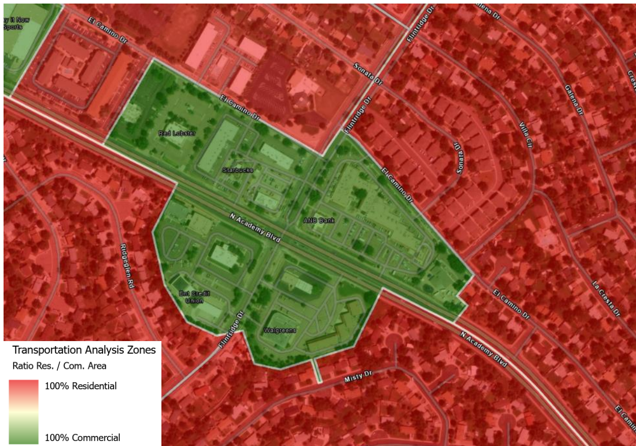
Figure 14: A detailed map of a 100% commercial TAZ surrounded by zones that are almost 100% residential, ensuring that all trips to and from the businesses in this zone are captured in the model
