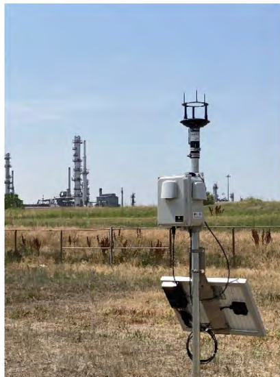
Figure 3. I-270 air quality sensor for research into the air quality impacts of construction activities.
