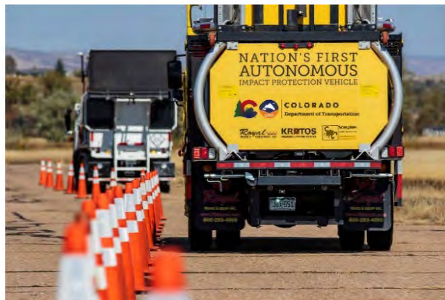
Figure 4. Autonomous attenuator truck testing. CDOT leads the Autonomous Maintenance Technology pooled fund study
